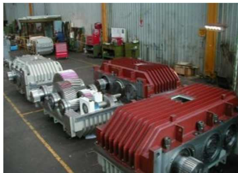
COAL CRUSHING GEARBOXES
