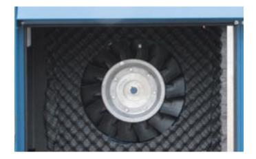
Regarding intake operation it is to be ensured that in case of separation filter damage, no combustible dust-air-mixture is sucked into the blower. For this reason, usually an additional filter element (emergency filter) must be provided by the unit design. This also means additional expenditures for the project work, assembly and installation.
